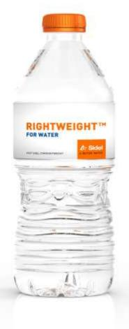
Bottle 7.95 gm Volume 500 ml Closure -1 gm Closure type 26/22 standard Top load 33 kg No Nitrogen dosing
