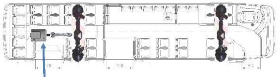
280 kW e-MOTOR The schematics of the main components is scaled to size. Battery/SuperCAP will be sized depending on further info regarding cycles and actual bus design in details. Will probably be splitted into multiple packs connected in series.
