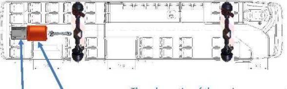
200 kW e-MOTOR 3 speed GEAR BOX The schematics of the main components is scaled to size. Battery/SuperCAP will be sized depending on further info regarding cycles and actual bus design in details. Will probably be splitted into multiple packs connected in series.
